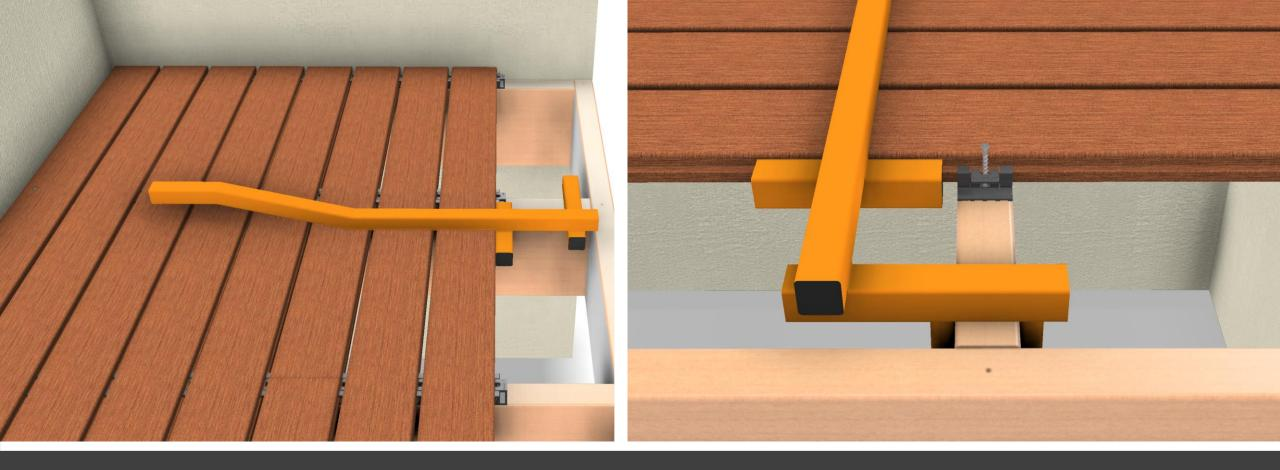
Step 9: If one of your boards is bowed, use a BoWrench to lock board into place. Then, place your clips just like in Step 7. Make sure to place board horned-side IN and use your BoWrench in the center of the board.
