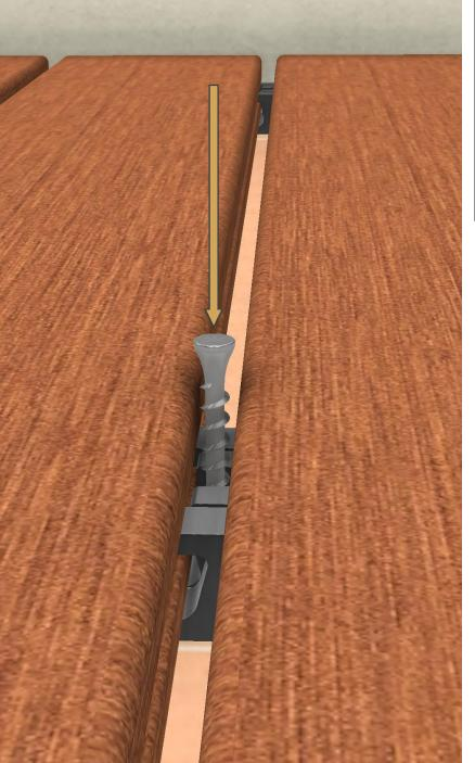
Step 11: Repeat Steps 7-9 until all boards are installed and fully fastened, except your last board.
