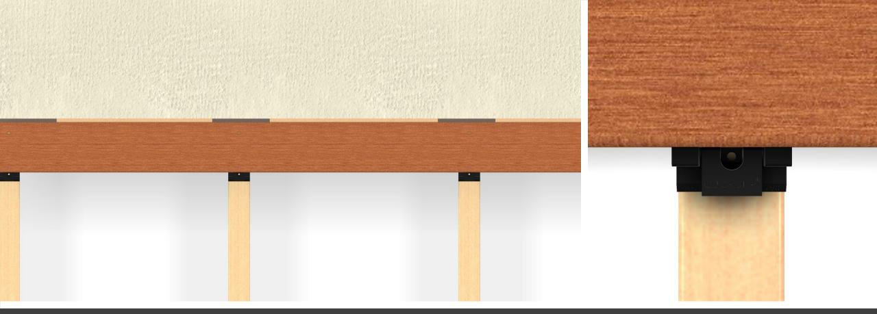
Step 3: Lay your first deck board down on top of the shim stock leaving approximately a 1/4" gap between the edge of the deck board and the structure. This allows room for swelling of the deck board.
