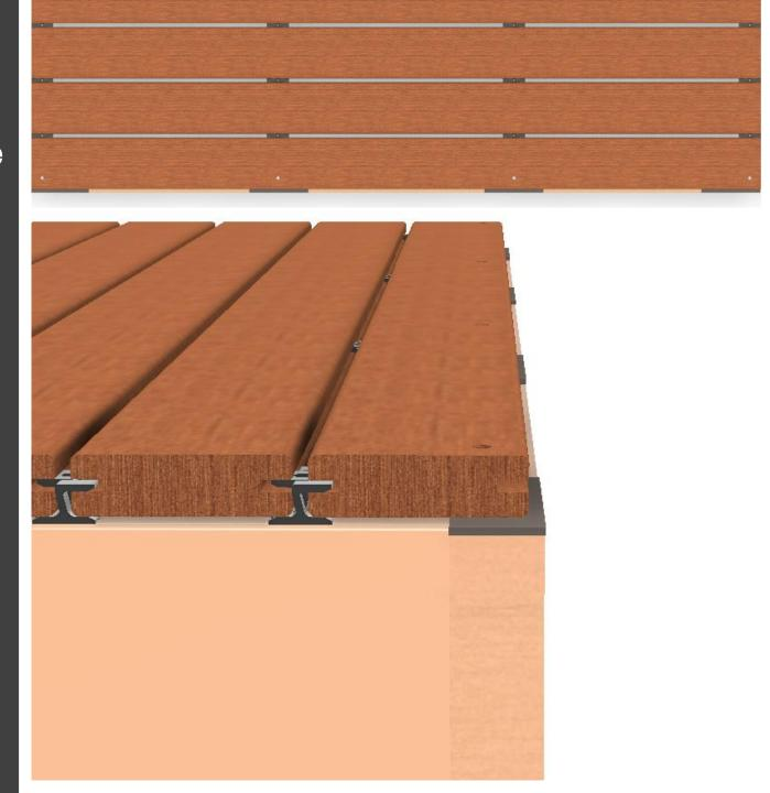
Step 16: (Optional) Create a beautiful finish to your deck by installing fascia boards of the same material as your deck boards. Be sure to leave a 1/4" gap to allow for swelling!
