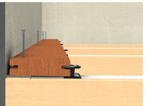
Step 5: Pre-drill your hole for a screw about two thirds to three quarters of the way up the width of the board. We recommend using a screw and plug system such as the PRO PLUG ® System by Starborn as this will give you the best looking finish, and seals the hole.
