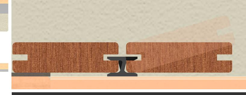
Step 7: Insert the next board, and then place clips on the open end. Remember to keep your center tab facing out. Repeat until you have about 5 boards with clips in place.
