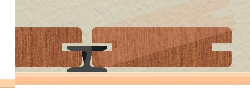
Step 5: Insert the next board, and then place clips on the open end. Remember to keep your center tab facing out. Repeat until you have about 5 boards with clips in place.
