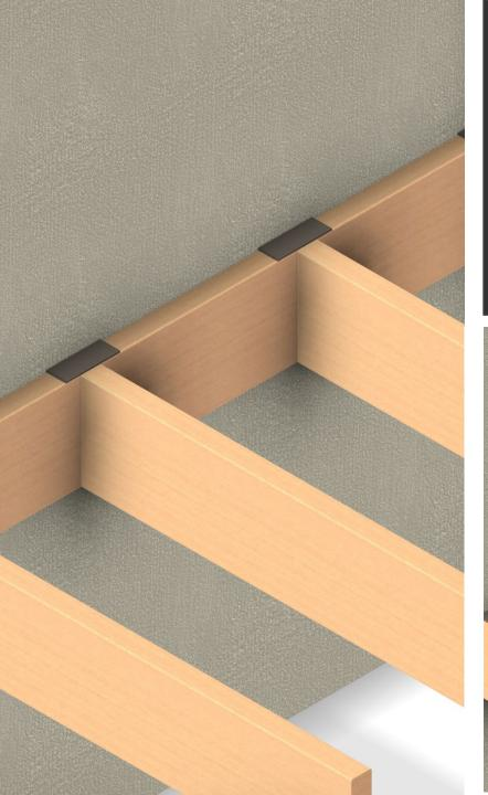
Step 1: Start on the side of the frame that is built off of your house or structure.
