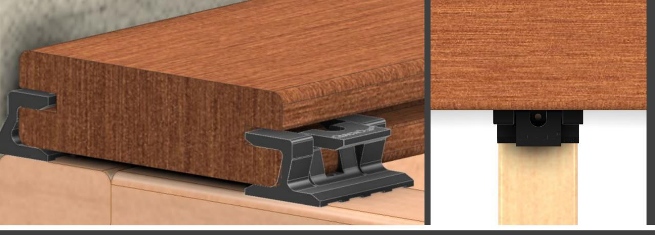
Step 3: Insert the starter clip into the groove of your first deck board which will leave approximately a 1/4" gap between the edge of the deck board and the structure. This allows room for swelling of the deck board.
