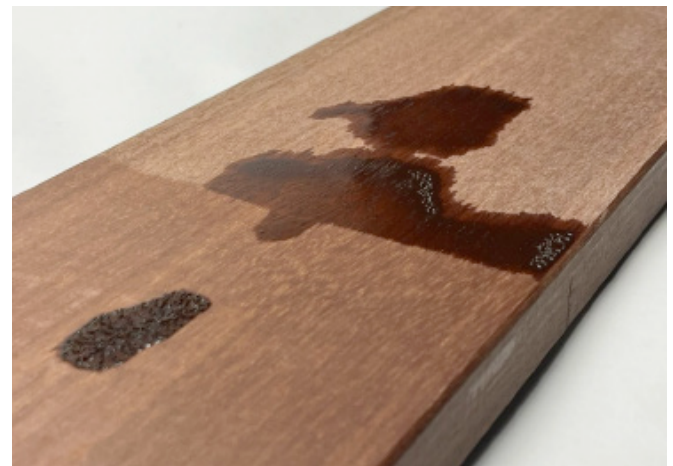
Torem Board, non-water popped (left), water popped (right)
