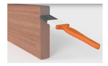
manufacturing to help prevent splitting and checking on the ends of boards. We require that the boards are end-sealed as soon as possible after making any cuts to the boards. A clear, water-resistant wax should be used. One such product is Anchorseal 2 from UC Coatings, although several other products are available. If the material is not end sealed the manufacturer will not honor any claims under the warranty.
