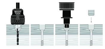
fastener look is the Starborn ProPlug system, as it still achieves face screwing for maximum hold-down and the use of stainless steel screws.
