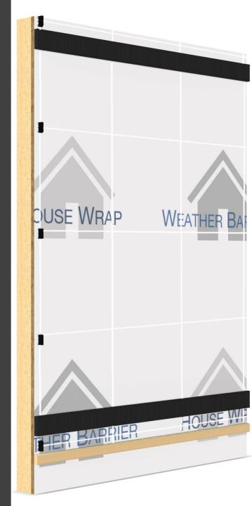
Step 9: Insert your first vertical board into the column of clips, gently tapping with rubber mallet if necessary.
