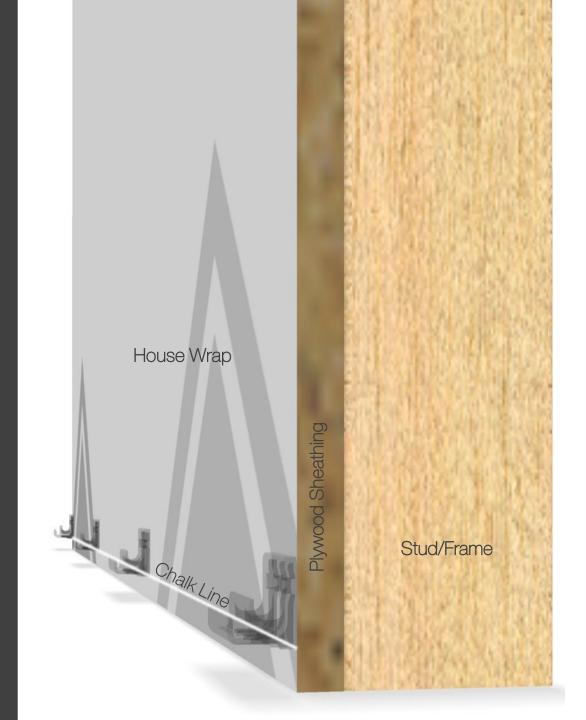
Step 3: Using a chalk line, mark where your studs are located for ease of installation.
