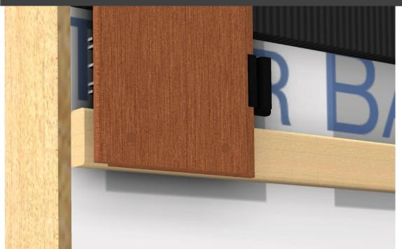
Step 11: Continue to install clips and Rainscreen boards repeating Steps 9 & 10 until you have covered the span of your installation area. Clips will usually require only one screw each at this point of installation.
