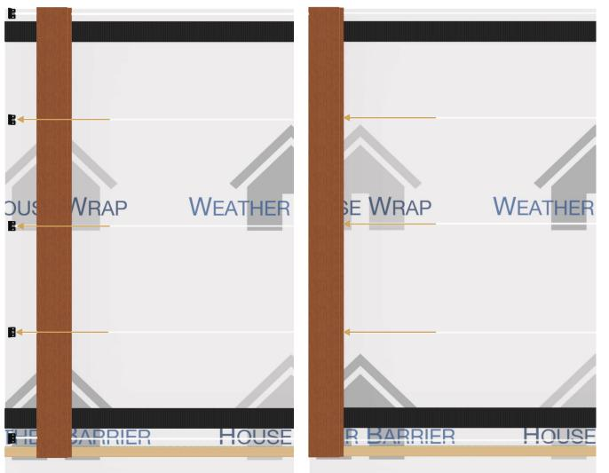
Step 10: Gently tap the bottom of the rainscreen board until it is flush with the furring strip. Fasten the board through the face with 2 screws. You will need to predrill the rainscreen board in order to face screw and avoid any splitting. We recommend using a screw and plug system for a seamless look.
