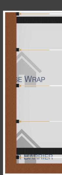
Step 16: Continue to install clips and Rainscreen boards until you have covered the span of your installation area. Clips will usually require only one screw each at this point of installation.
