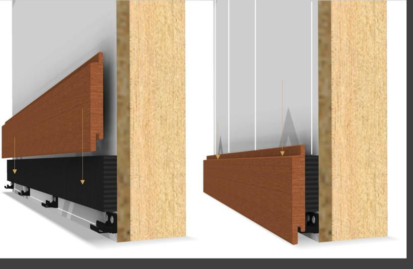
Step 7: Install the first Nova Rainscreen Siding board on top of the starter clips.
