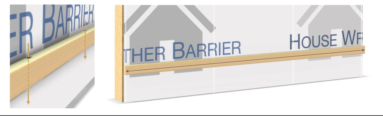
Step 4: Obtain enough length of 1 x 2" furring strips to cover the entire length of the wall. Cut small vertical channels (weep holes) into the furring strip approximately 12 inches apart. These are required to allow for drainage through the furring strip. These channels will face the wall.
