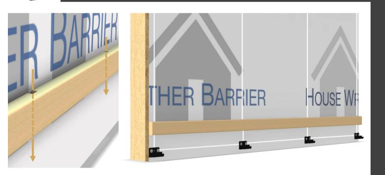
Step 8: Fasten the furring strip across the length of the wall above the installed starter clips to the appropriate height that matches the width of the trim board. Ensure the furring strip is installed into the framing
